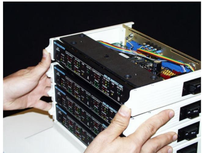
To remove Lincs, **push up on the thumb tab** as shown to apply upward force properly (from the front of the Linc). **Lifting from the back of the Linc will bend the jacks.**
